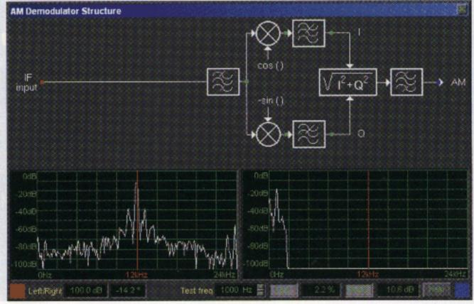
This is very useful in crowded shortwave broadcast bands if one sideband is damaged by neighbouring interference. Simply turn the damaged sideband off using USB or LSB instead and the signal clarity improves dramatically.
