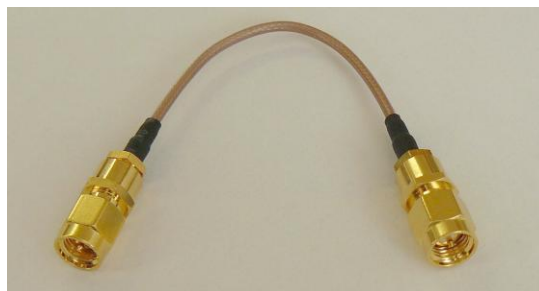
Picture 2-9: SMA interconnect cable for frequency reference
