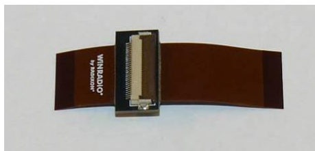
Picture 2-7: Digital synchronization cable for the WR-G35DDCi receiver
