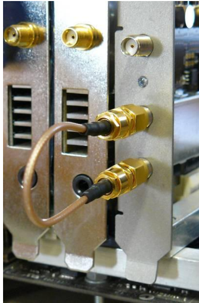
Picture 3-9: Installing the frequency reference SMA interconnect cable for internal frequency operation
